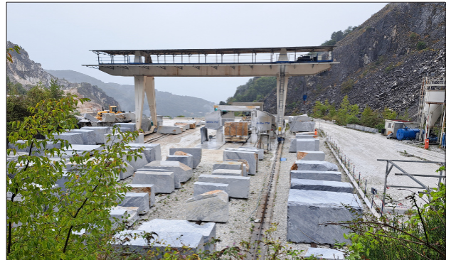
Crane on tracks for shifting marble blocks
